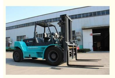
DIESEL 15 TON FORKLIFT LIFT CAPACITY: 15 TONNE LIFT HEIGHT: 3M TO 7M FUEL TYPE: DIESEL
