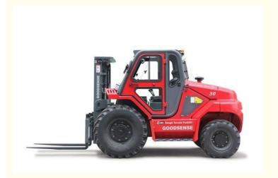
THE EXCELLENT WEIGHT DISTRIBUTION GIVES THE FORKLIFT GREAT STABILITY. THIS CAN BE SEEN IN THE SMOOTH DRIVE AND THE EASE WITH WHICH IT CAN BE MANOEUVRED. ALSO, THE DRIVER CAN SEE THE LOAD AT ALL TIMES REGARDLESS OF ITS POSITION. THE FRONT GLASS AND THE WAY THE MAST IS POSITIONED BOTH PROVIDES GREAT VISIBILITY TO THE DRIVER.
